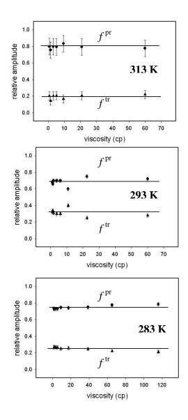
**Fig. S3.** Independence of solution viscosity of the relative amplitudes  $f^{\text{pr}}$  and  $f^{\text{rr}}$ , respectively, of the electron-transfer reaction occurring within persistent (•) and transient (•) protein complex in Scheme S1 at different temperatures. Viscosity of the sodium phosphate buffer solution at pH 7.0 and ionic strength 10 mM was adjusted with glycerol.
